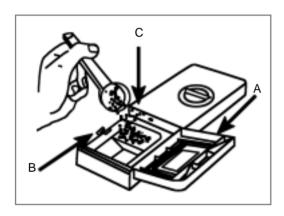
Notice:To facilitate closing the cover, remove any excess detergent on the edges of the dispenser.
